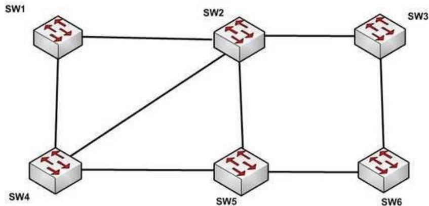
STP probes the network at regular intervals to identify the failure or addition of a link, switch, or bridge. In the case of any topology changes, STP reconfigures switch ports to prevent loops. The end result is one active Layer 2 path through the switch network.
